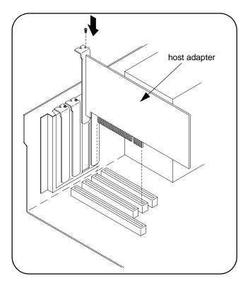
Figure 2-4. Installing the Host Adapter.
