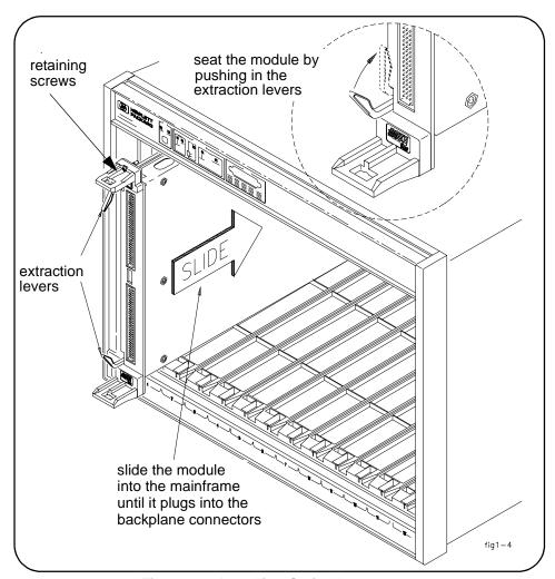
Figure 2-8. Installing C-size Instruments.
