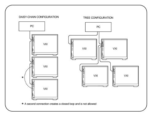
Figure 2-7. IEEE 1394 Interface Configurations.
