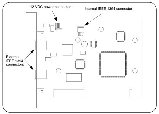
Figure 2-1. Layout of the Adaptec® AHA-8940 1394-to-PCI Host Adapter.
