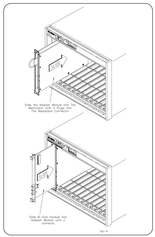
Figure 2-9. Installing A- and B-size VXI Instruments.
