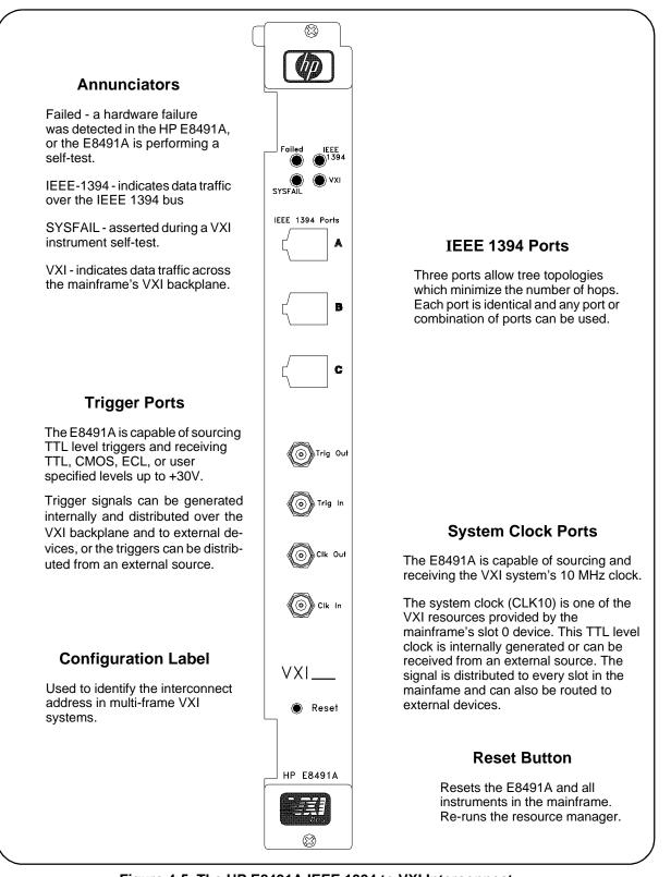
Figure 4-5. The HP E8491A IEEE 1394 to VXI Interconnect.
