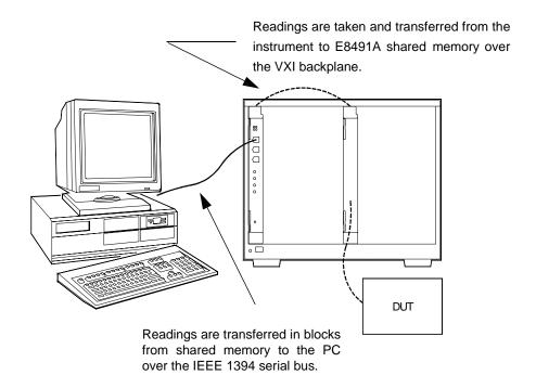
Figure 3-4. Storing Readings in Shared Memory.
