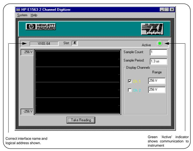
Figure 2-15. Soft Front Panel Indicating PC - Mainframe Communication.
