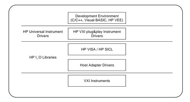
Figure 4-6. System Software and Drivers.
