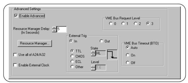
Figure 3-1. Configuring the HP E8491A External Trigger Ports.
