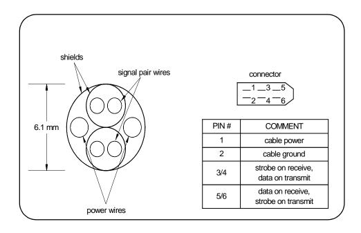
Figure 4-4. Cross-section of the IEEE 1394 Cable.
