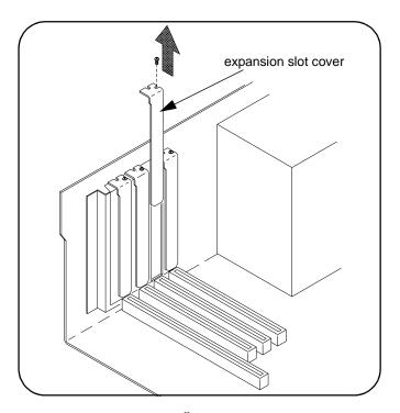
Figure 2-3. Removing the PC Expansion Slot Cover.
