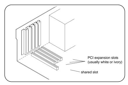
Figure 2-2. Locating a PCI bus Expansion Slot.
